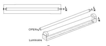
5 Install LED tube and Earth (Ground)
